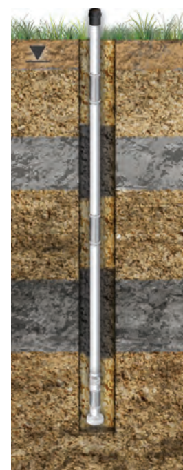
Typical 3 or 7-Channel CMT Installation using Layers of Bentonite and Sand Backfilled from Surface
